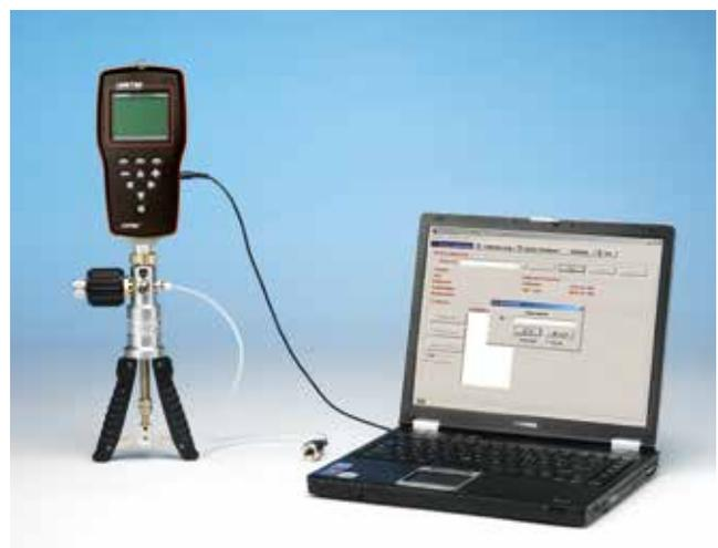
Setup with JOFRA HPC system B connected to a PC with JOFRACAL
