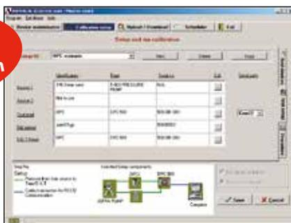
JOFRACTAL integrates with JOFRA calibration instruments. As for temperature calibrators, it is the whole range of temperature calibrators. Regarding pressure calibrators, it integrates with DPC-500, HPC and IPI pressure calibrators. JOFRACAL also has full integration with the series of signal calibrators.
