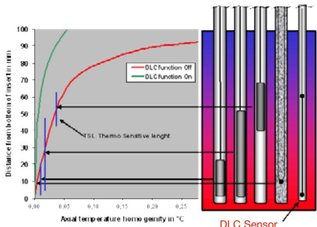
Axial temperature curves for an RTC calibrator with and without the DLC functionality activated. DLC controlling is automatically disabled when the stirrer is started.
