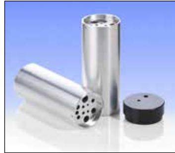
These inserts have holes for both the DLC and two reference sensors (4 mm and 1/4"). These holes are marked for correct use.
