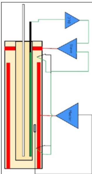
The new DLC sensor improves the homogeneity even more by controlling the homogeneity not only in the well, but also inside the insert, where the sensors-under-test are placed during calibration. The DLC sensor measures the temperature homogeneity in the insert and provides feedback to the active dual-zone system, which now compensates the temperature difference to a minimum inside the insert. In this way, the DLC function makes the homogeneity independent of the different loads of the insert.
